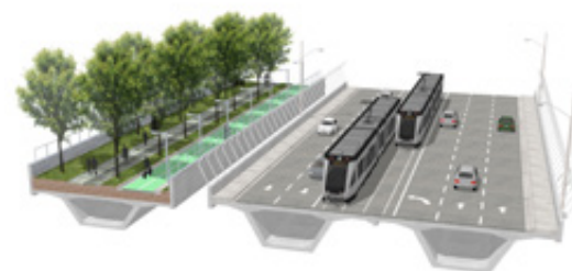
Alternative 1 - Maintains existing bridge and adds a new adjacent bridge with sidewalk, dedicated two-way cycle track, and landscaping.
