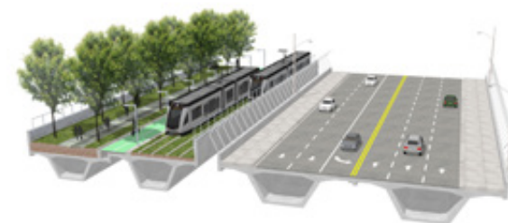
Alternative 2 - Maintains existing bridge and adds a new adjacent bridge with sidewalk, dedicated two-way cycle track, landscaping, and transit.
