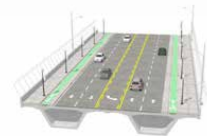
Alternative 3 - Maintains existing bridge, but retrofits it in order to make room for protected bike lanes
